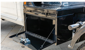
Two lockable integrated toolboxes featuring T-handle compression latches.
