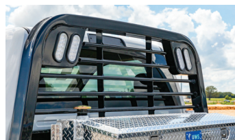
Integrated single-piece headache rack with optional cargo light and standard integrated rear LED lighting.
